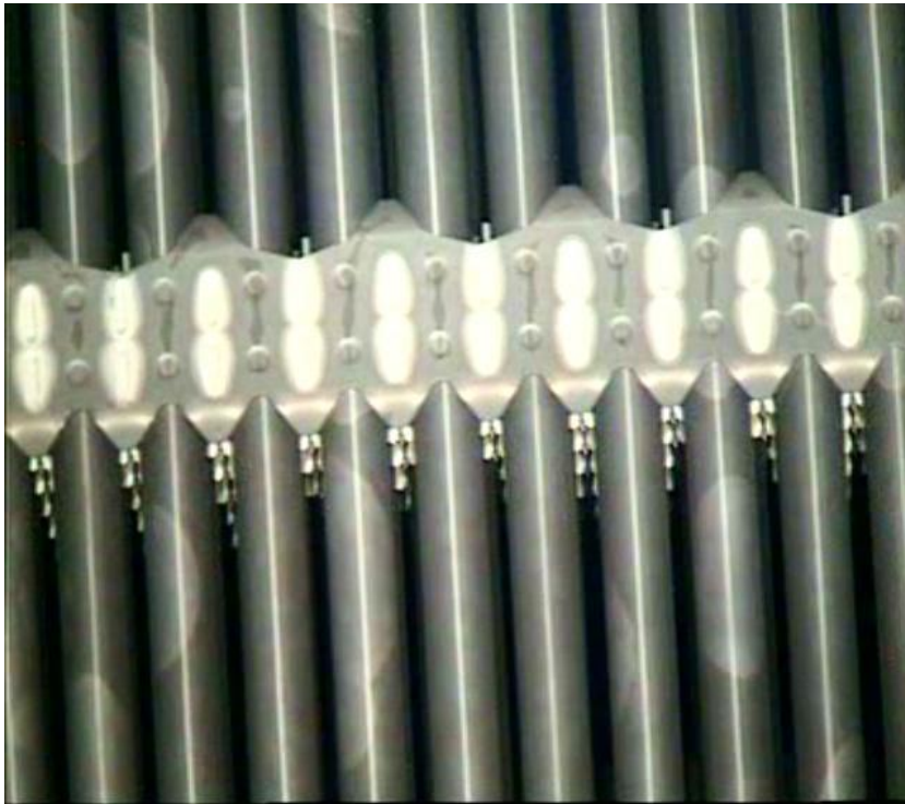
Examining the underside of a mid-span mixing grid
